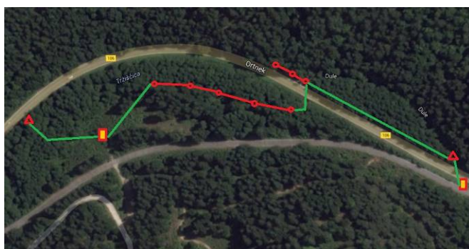
Figure: Dynamic traffic signs Ortnek; sensors (red line), power lines (green line), solar cells (yellow rectangle) and traffic signs (triangle).
