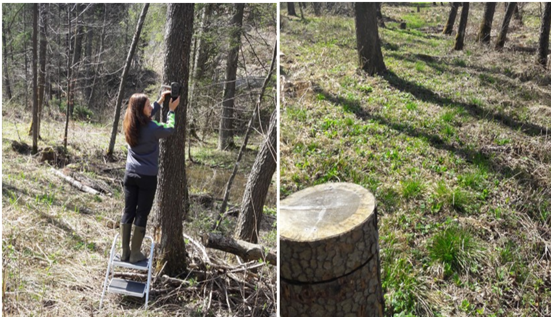
Figure: Installation of IR cameras at Ortnek and sensors in wooden stumps capable to detect large animals approaching the roadway (photo: Z. Pavšek).
