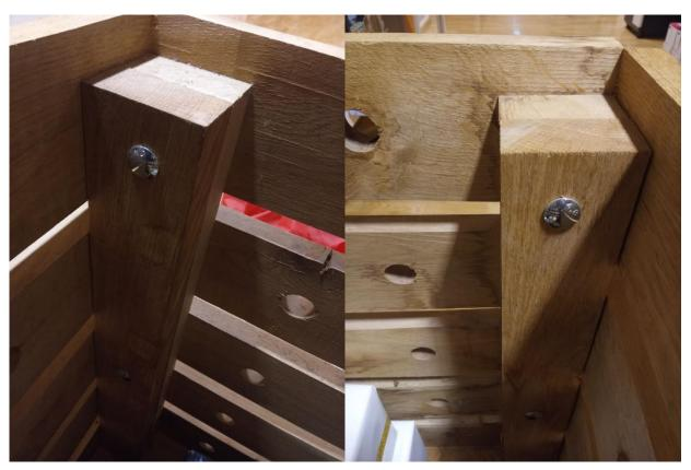
2. Attach a metal plate to the bottom of each corner with a single wood screw (6 x 120, TX 30). The tile serves to attach the composter to poles driven into the ground (see point 5), and it is easiest to install them before installing the compost lid, which significantly increases the weight of the composter.
