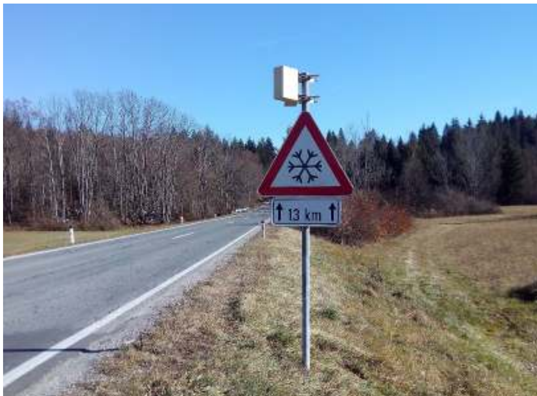
Figure 10: Traffic counter placed on the pole of traffic sign near Dolenja vas (Jasnica).
