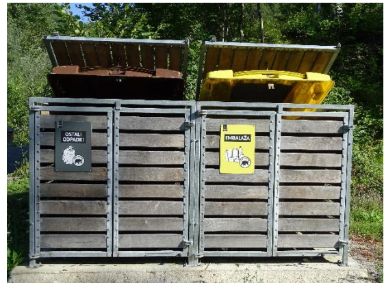
Figure 25: Flawless operation of “bear-proof” garbage housings for large (~ 1000 litre) containers.
