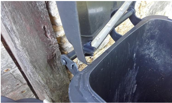
Figure 4: Broken cover of individual garbage can.
