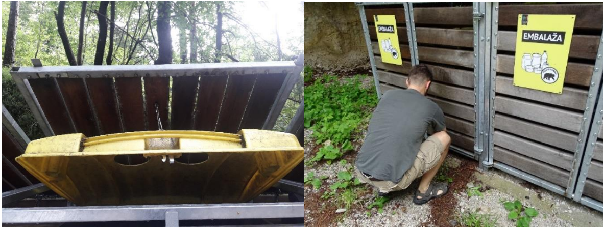
Figure 1 and 2: Good operation of the “bear-proof” garbage housings for large (~ 1000 litre) containers.
