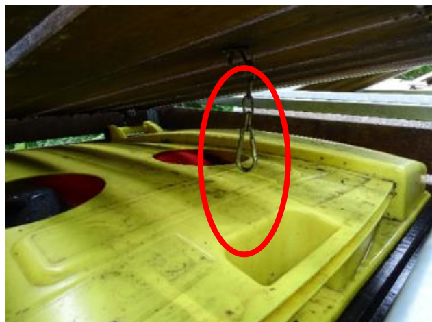
Figure 6: Missing cover pin of the newly replaced container.
